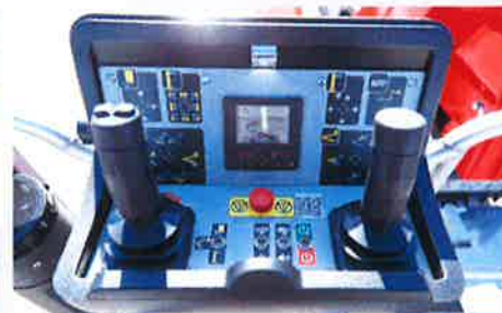
FPC: Full proportional CANbus controls with display
