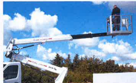
Cage rotator: 2 x 90°
