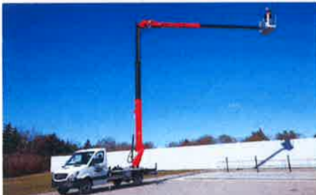
Perfectly vertical lower boom and horizontal upper boom**
